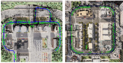
Figure 6: The examples of the maps in Traffic Congestion dataset and the outputs of GSLAMOT. Blue points represent ego-motion trajectories, green boxes represent tracklets, and black points represent map points.
