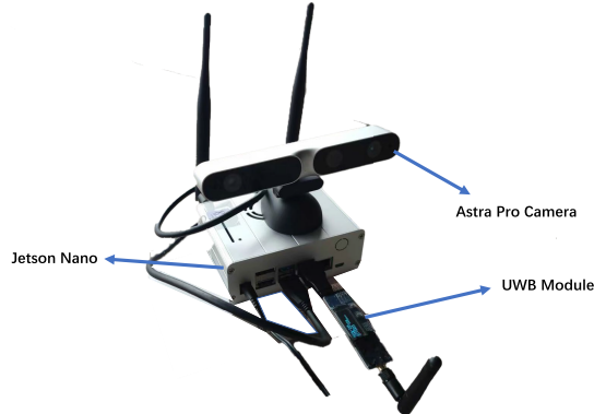
Fig. 15. The node containing a Jetson nano, UWB module, and Astra Pro camera.
